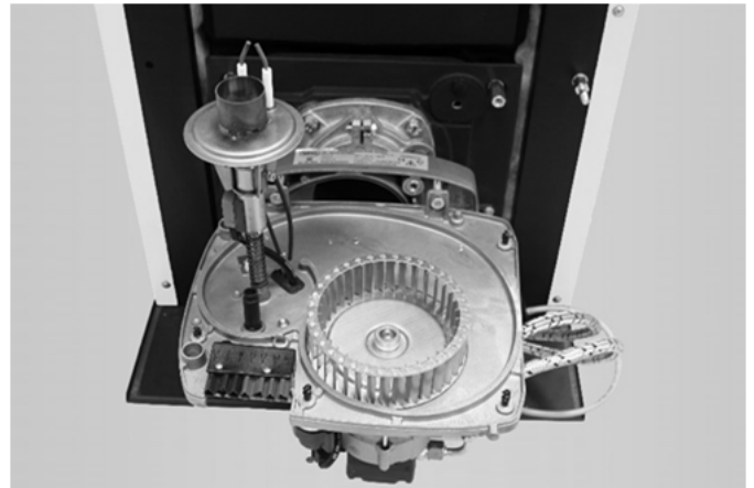
Abb. 22: Brenner in Serviceposition
