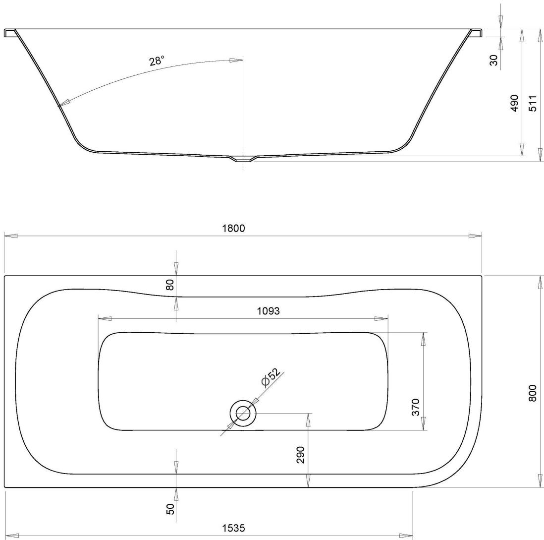
FORMAT Design Sonderform Ecke links Einbauversion 1800x800
