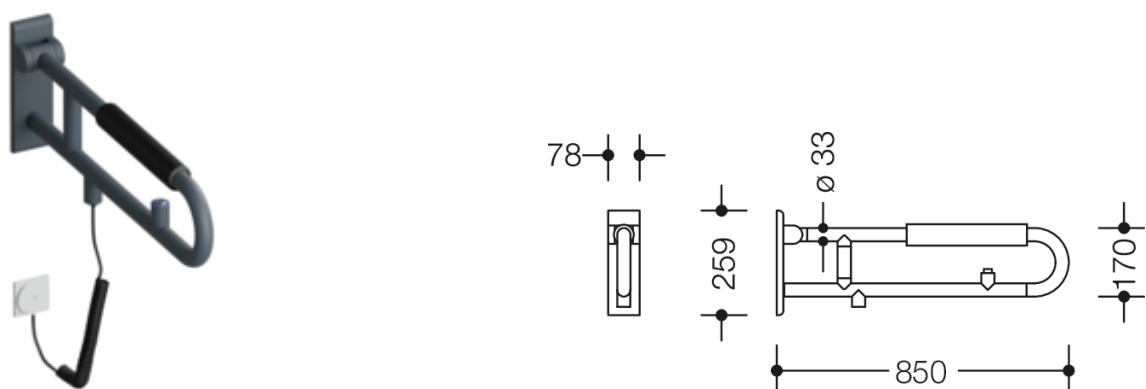
Abmessungen in mm
