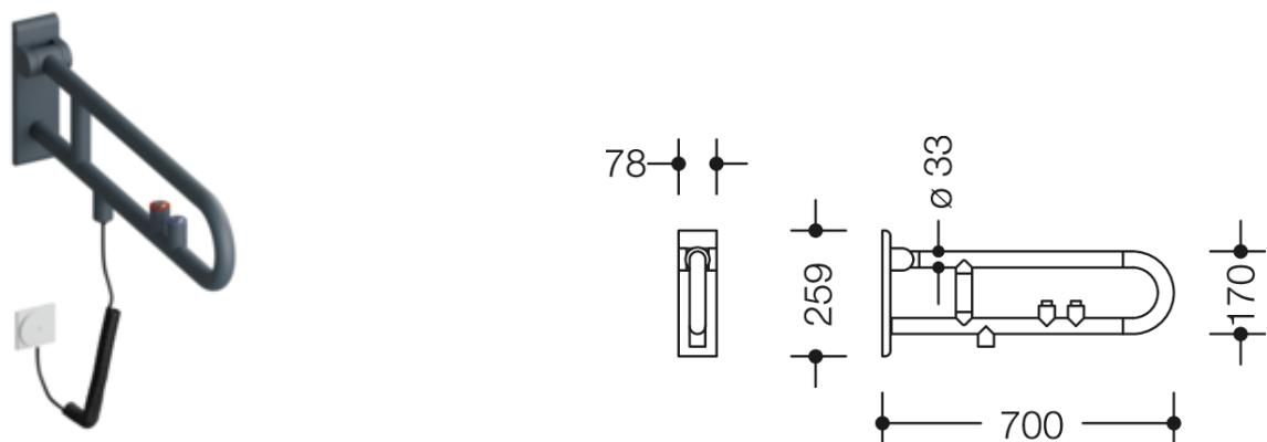
Abmessungen in mm
