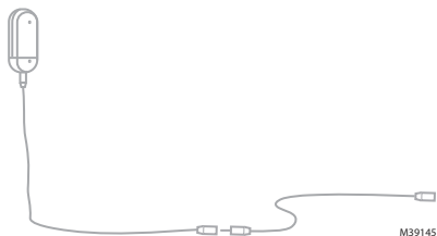
Fig. 1. Plugging in additional cable sensors.
