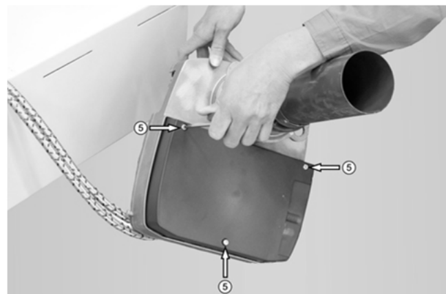
Fig. 2: Removing the intake silencer
